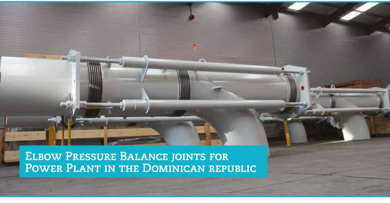
MACOGA has successfully designed, manufactured and tested Elbow **Pressure Balanced Expansion Joints to** be installed in the Punta Catalina Power Plant for Corporación Dominicana de Empresas Eléctricas Estatales (CDEEE) in the Dominican Republic.
